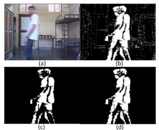
Fig.6 Current frame (a), Image Thresholding (b), Erosion Operation (c) and Dilation Operation (d)
