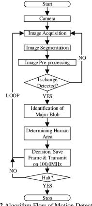
Fig.2 Algorithm Flow of Motion Detection
