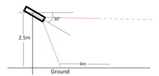
Fig.8 Camera installation for obtaining the best results
